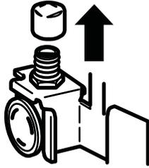
Place the compression nut and ferrule (sleeve) onto the end of the tubing.
